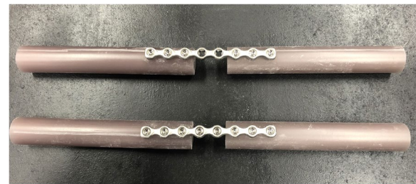
Fig. 1 Plate constructs without (top) and with (bottom) locking plugs
