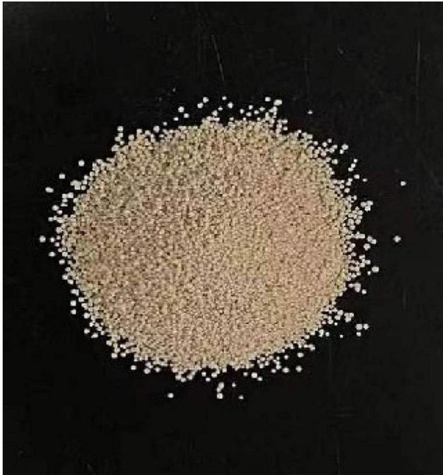
**Fig. 1** Prepared cinnamon oil and star anise oil compound essential oil pellets
